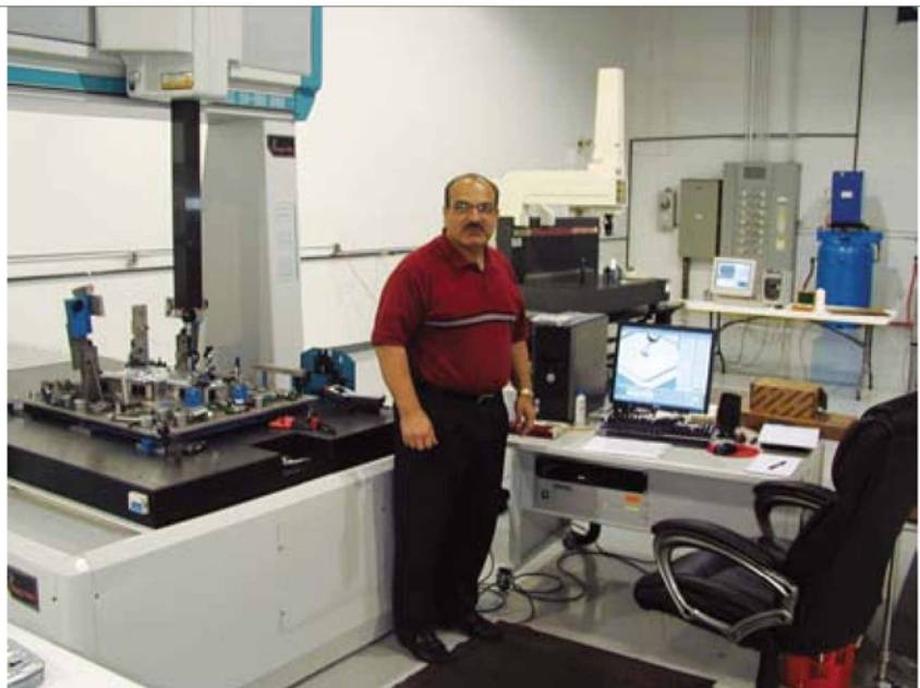
Dimensional Measurement's owner Mohamed Abdelhafiz with his new Wenzel LH8.10.7 CMM. The Sheffield RS150 can be seen in the background. Source: Xspect Solutions Inc.
